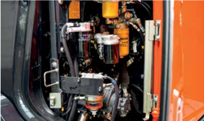
Convenience access to all filters in one compartment.
