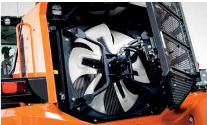
Intelligent fan operation system prevents radiators clogging.
